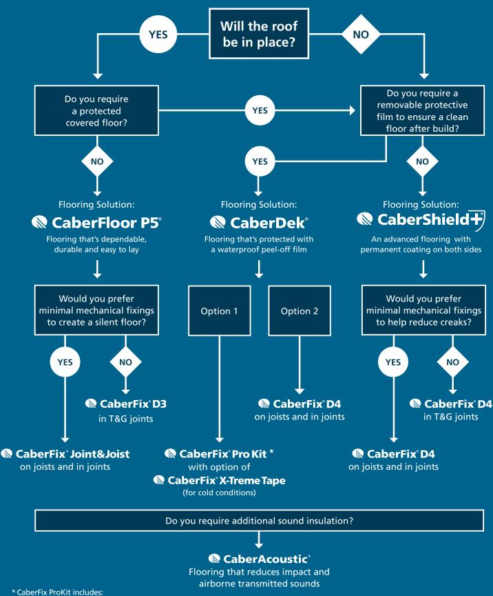
\* CaberFix ProKit includes: 1 × CaberFix D3, 7 × CaberFix Joint&Joist, 3 × CaberFix Tape
